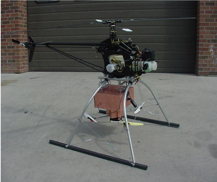
Figure 2: Bergen helicopter complete with frame modifications
