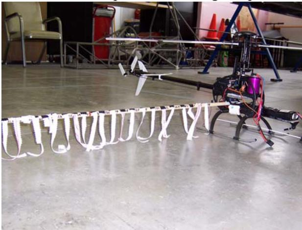
Figure 5.1: Logo electric helicopter equipped with rotor wash analysis boom.
