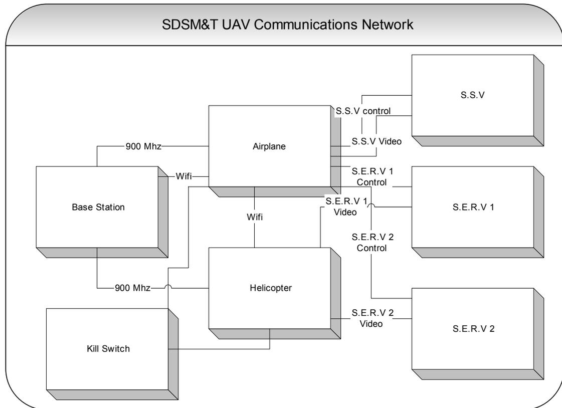
Figure 1.2: UAV communication network
