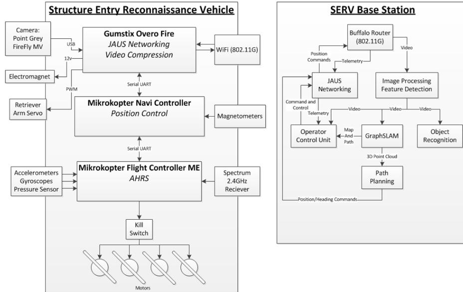
Figure 1: 2010 SDSM&T System Architecture
