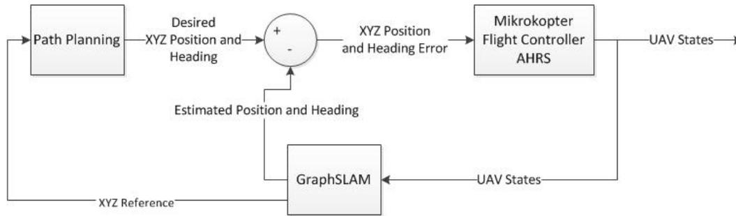
Figure 4: *SDSM&T Developed Control Block Diagram*
