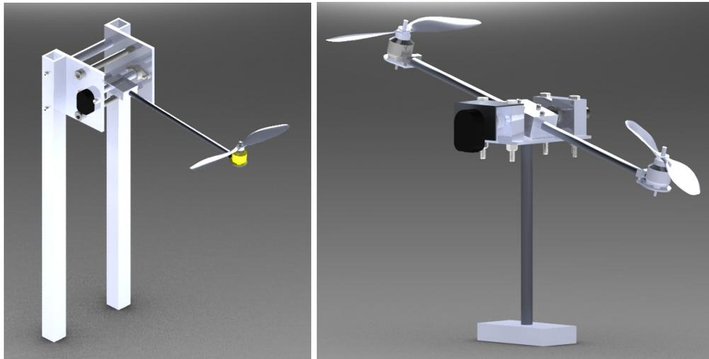
(a) Rotor Pendulum Test System
