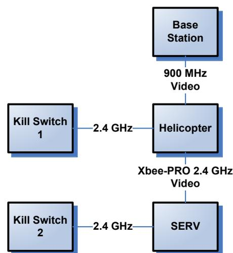
Figure 1. UAV System Architecture
