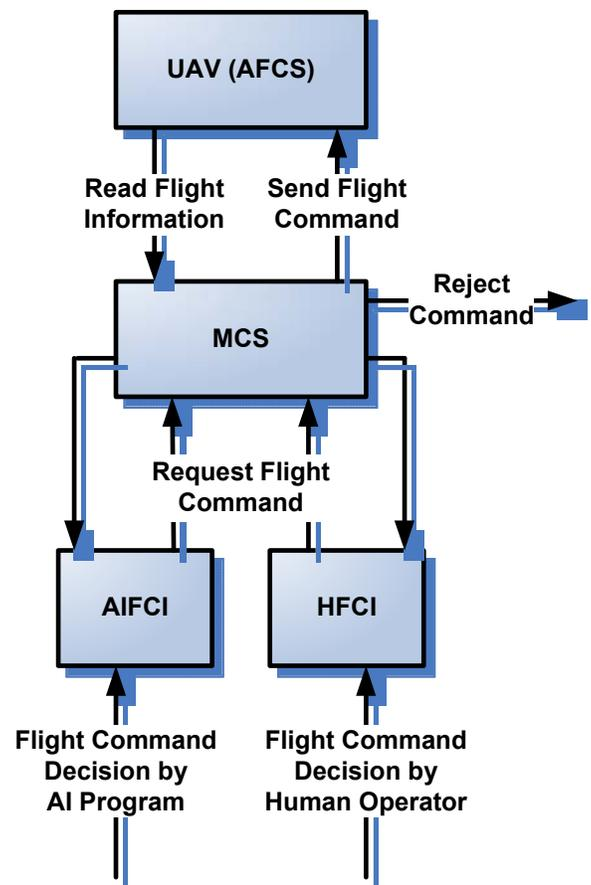
Figure 2. Control System Architecture
