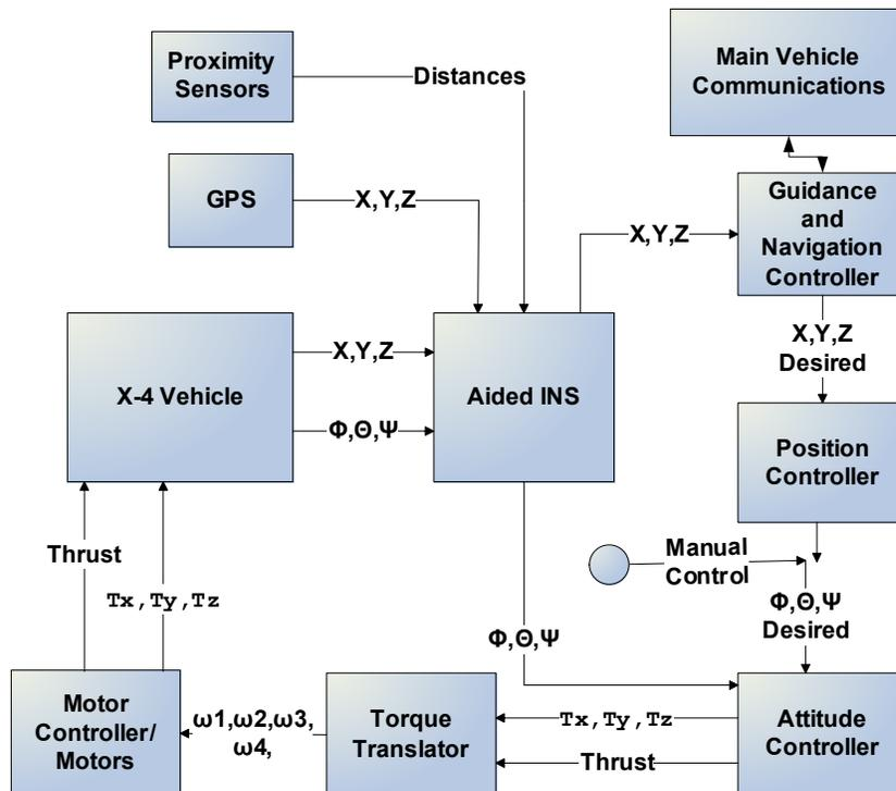
Figure 4. SERV Control Diagram
