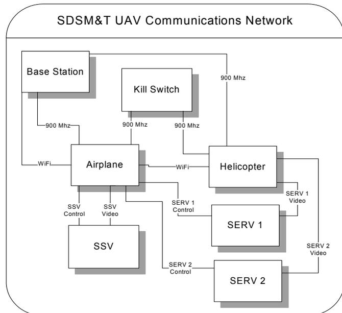
**Figure 1:** UAV Communications Network Diagram
